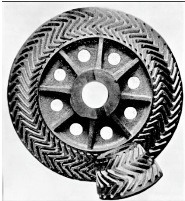
Herringbone bull and pinion bevel gears showing complex gear tooth patterns Credit: Wikipedia Commons
