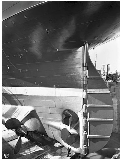
Titanic's sister, Olympic, showing port wing and center turbine propellers and rudder. Credit: Wikipedia
